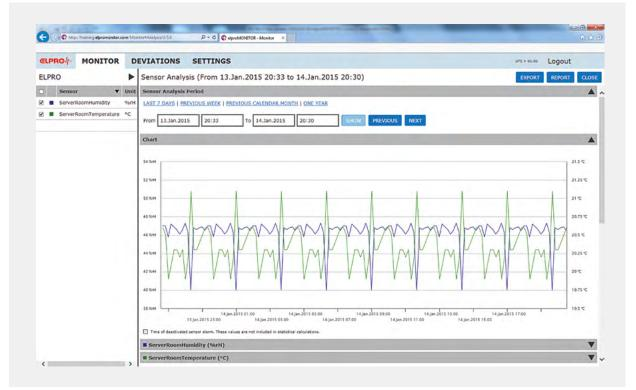
Centralized database software such as elproMONITOR (shown above) enables quick, easy, and secure analysis of temperature excursions, reporting, and data archival for rooms, refrigerators, freezers, and cryogenic and ultra-low containers.
